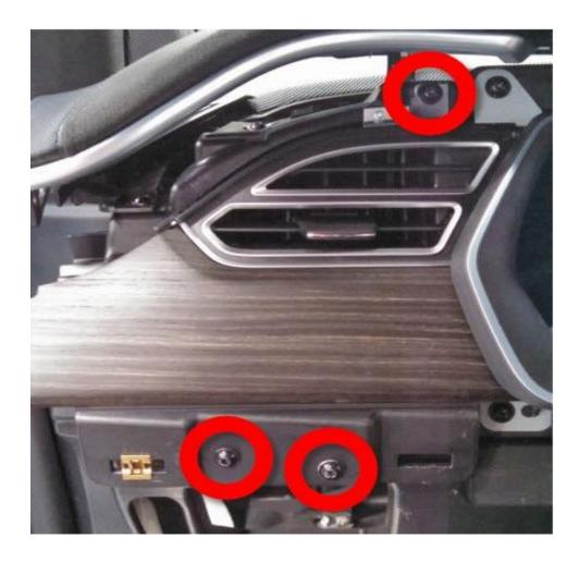
4. Remove the inner face level vent from the vehicle.
