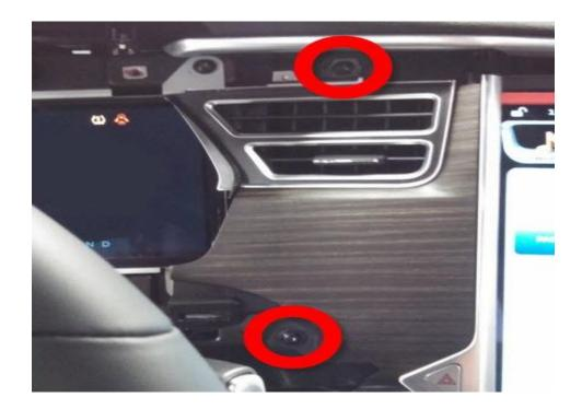
5. Remove the fixing screws (2 pcs) between the top pad and the instrument panel carrier (torque 1.2 Nm).
