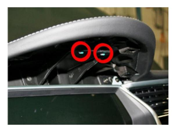
6. Release the fixing clips (2 pcs) between the steering column cover and the instrument cluster frame.
