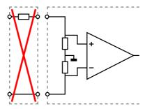
Instead a differential attenuator with attenuation in both signal paths is required.
