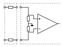
A differential input also means that both sides of the input have a high impedance. There is no connection to ground as in conventional oscilloscopes which are used with coax cables. Using a coax cable on the Handyscope HS6 DIFF would result in the instrument picking up a lot of external interference.
