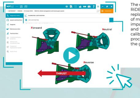
The electronic braking control system RiDE requires calibration after component replacement or even after an impact capable of misadjusting the gate mechanism. These impacts are pretty common during docking and transport of the jet ski on ground. The calibration consists in an automatic learning process of the upper and lower values that the gate might reach.
